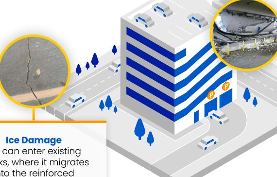
Ice can enter existing cracks, where it migrates into the reinforced concrete slab, causing delamination or fractures.
